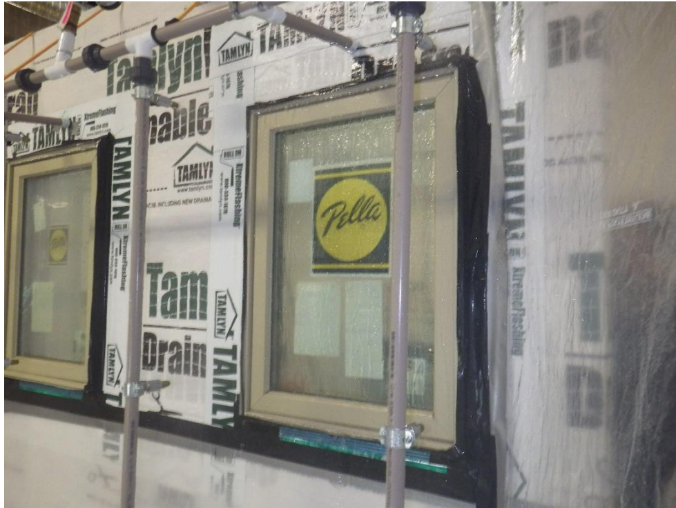
Photograph 15: Specimen B - Water penetration resistance test
