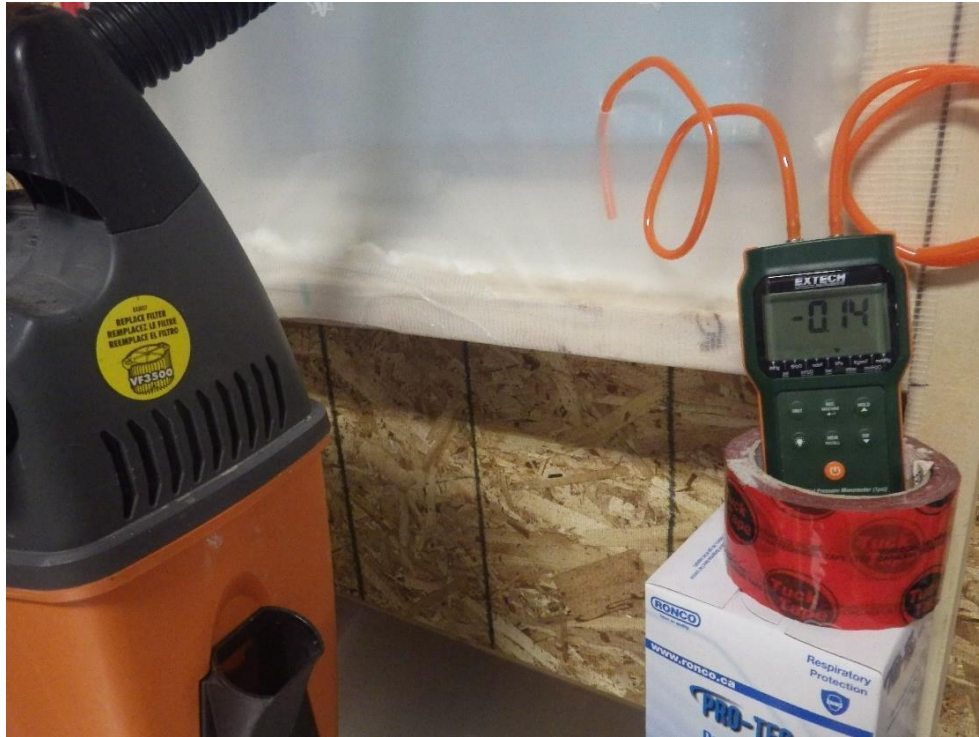
Photograph 19: Specimen A with interior seal Water penetration resistance test
