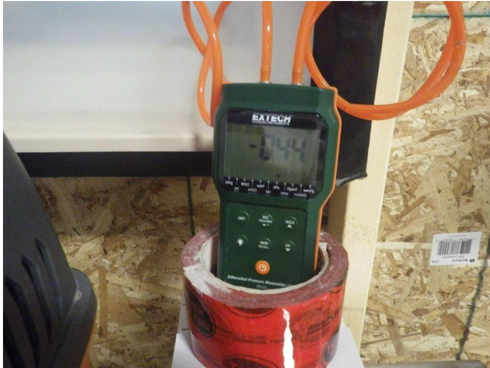
Photograph 21: Specimen B with interior seal Water penetration resistance test
