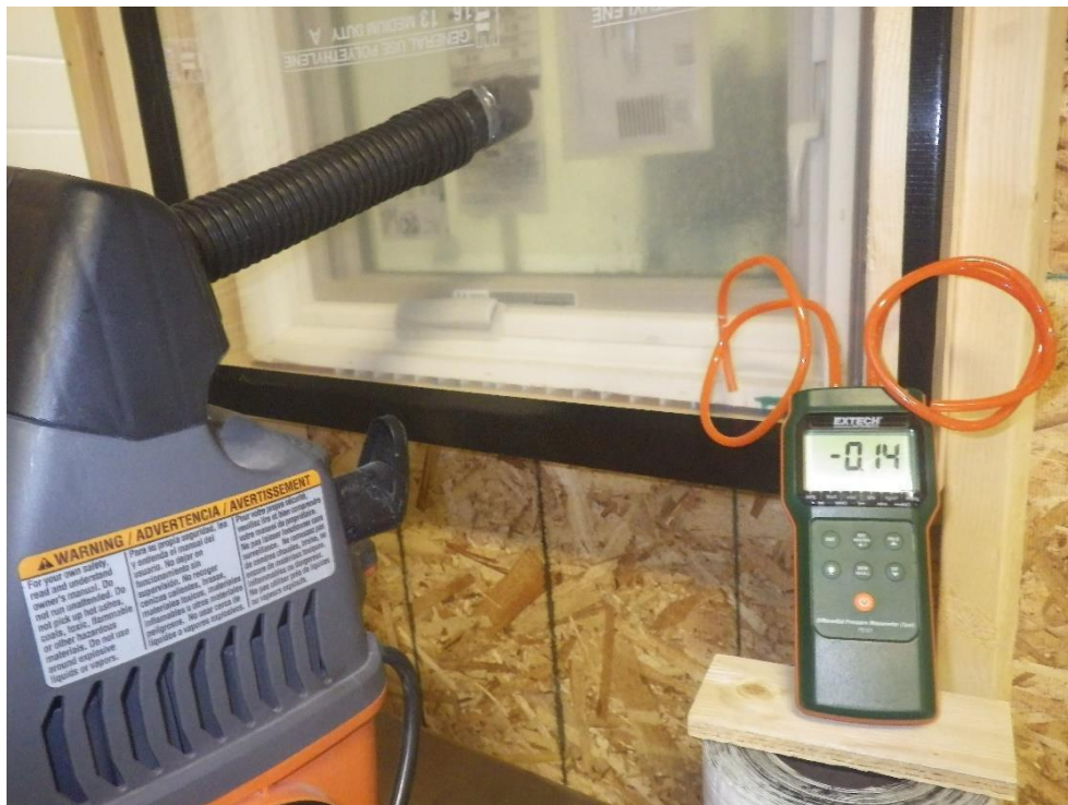
Photograph 16: Specimen B - Water penetration resistance test
